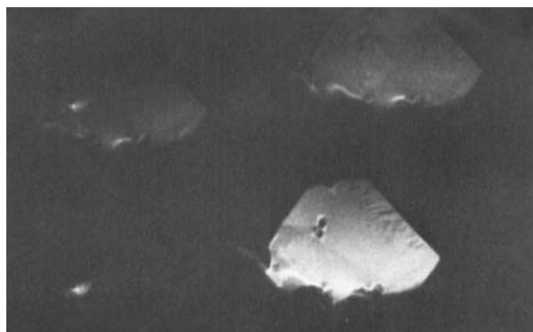
FIGURE 5. Synchrotron topograph of a macroscopic DSP crystal in the Laue geometry
